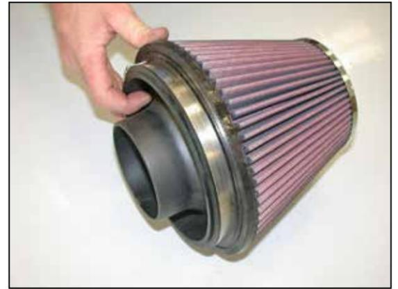
19. Install the radiused filter adapter into the K&N® air filter as shown. Secure with the provided hose clamp.
