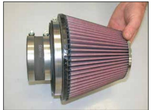
20. Install the provided silicone hose (08630) onto the filter adapter and secure with the provided hose clamp as shown.
