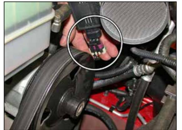
6. Release the mass air sensor electrical connection clip, then disconnect the electrical connection.
