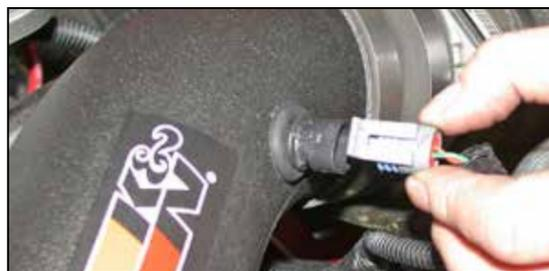
31. Reconnect the temperature sensor electrical connection.
