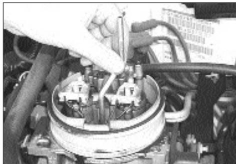
6. Install the provided Z stud into the threaded hole located just in front of and between the two throttle ports, then screw down completely.
