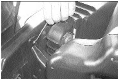
2. Loosen and remove the hex bolt that secures the air inlet to the radiator support.
