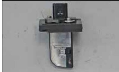
20. Install the mass air sensor into the K&N® sensor adapter as shown. Secure with the provided hardware.
