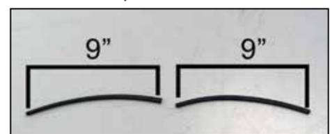
9. Cut the provided edge trim into two 9" sections as shown.
