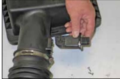
19. Remove the two screws securing the mass air sensor and then remove the mass air sensor from the stock intake tube as shown.
