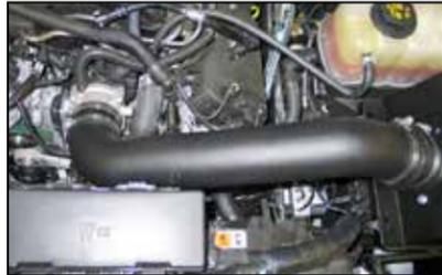
22. Install the K&N® intake tube assembly into the silicone hose at the filter adapter and then into the silicone hose on the throttle body and secure with the provided hose clamps.
