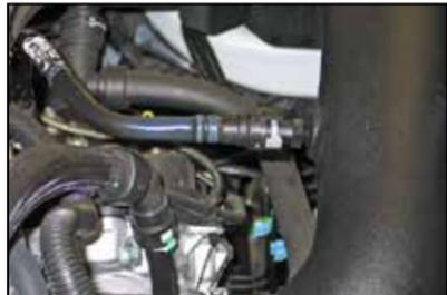
23. Connect the crankcase vent hose to the quick disconnect fitting in the K&N® intake tube.
