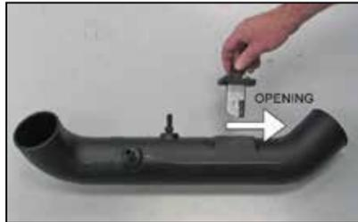
21. Install the mass air sensor assembly into the K&N® intake tube and secure with the provided hardware.
