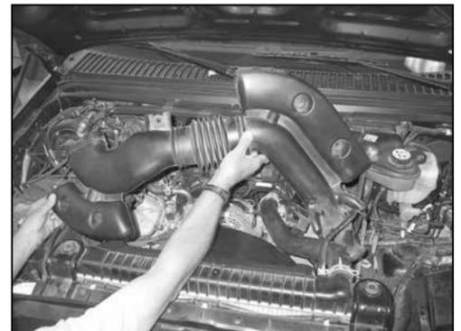
5. Unhook the factory fresh air tube from stock air box and radiator core support. Then remove the fresh air tube from the vehicle.
