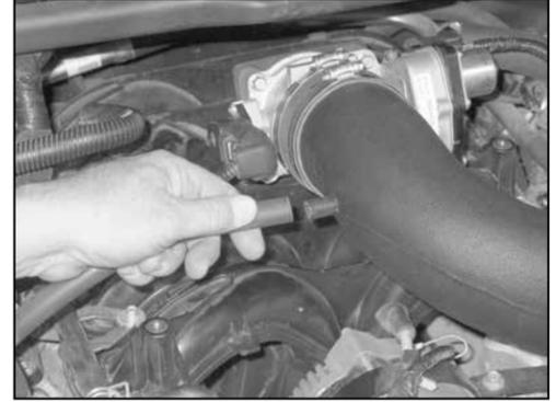
34. Install the supplied crank case vent hose onto the valve cover fitting and then onto the K&N® intake tube as shown.
