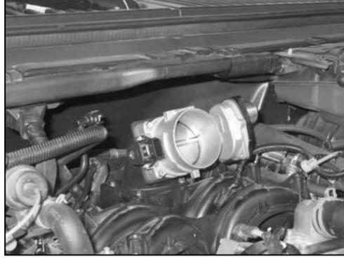
13. Install the throttle body assembly onto the intake manifold with the provided hardware as shown.
