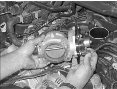
11. Lift the throttle body from the intake manifold. Then disconnect the throttle body motor electrical connection.
