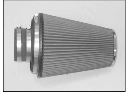
36. Install the filter adapter assembly into the K&N® filter and secure with the provided hose clamp.
