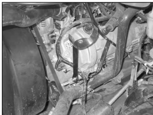
17. Install the tube mounting bracket assembly onto the threaded stud with the spacer installed in step #15. Then secure with the provided hardware.
