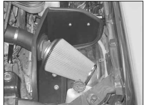
37. Install the filter adapter assembly into the K&N® filter and secure with the provided hose clamp.
