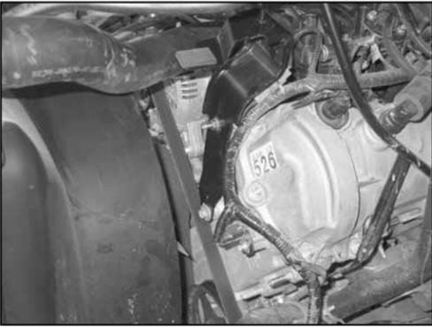
8. Remove the bolt and nut that secure the mounting bracket for the stock fresh air intake tube and then remove the mounting bracket.
