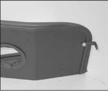
23. Install the small "L" bracket (010060) onto the heat shield as shown with the provided hardware.
