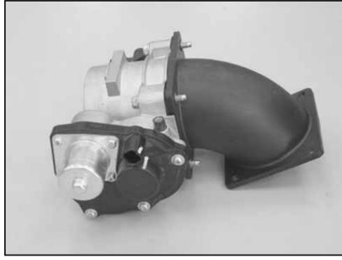
12. Using the factory mounting bolts from step #10, secure the throttle body to the K&N® throttle body adapter with the gasket as shown.
