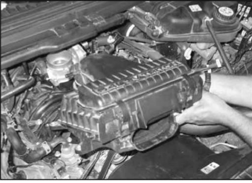
7. Remove the factory air box from the vehicle.
