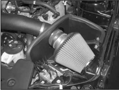
25. Install the air filter assembly onto the K&N® intake tube as shown and secure with the provided hose clamp.
