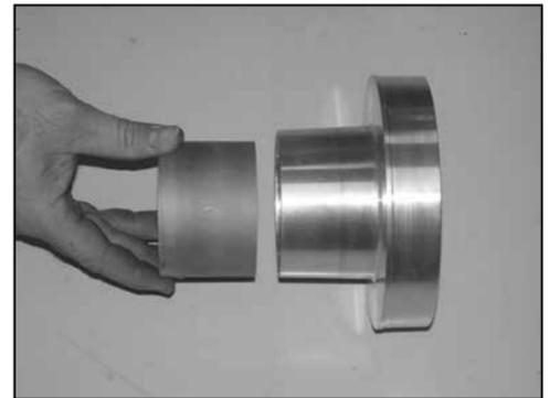
22. Vehicles that come equipped with Hydrocarbon trap, place the Hydrocarbon trap into the filter adapter as shown.
