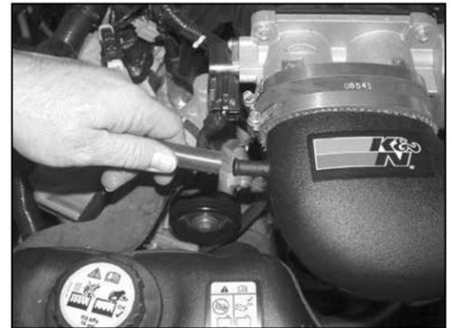
20. Install the supplied vent hose onto the vent port on the valve cover and secure with the provided hose clamp, then onto the K&N® intake tube as shown.
