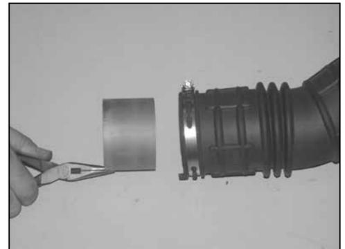
21. Vehicles that come equipped with Hydrocarbon trap, use a pair of needle nose pliers, to remove the Hydrocarbon trap from the stock intake tube as shown.
