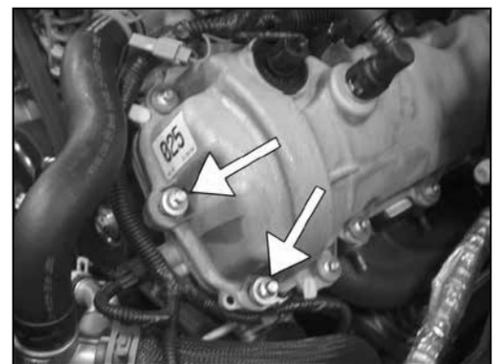
8. Remove the two valve cover bolts shown. **NOTE: These bolts will be reused.**
