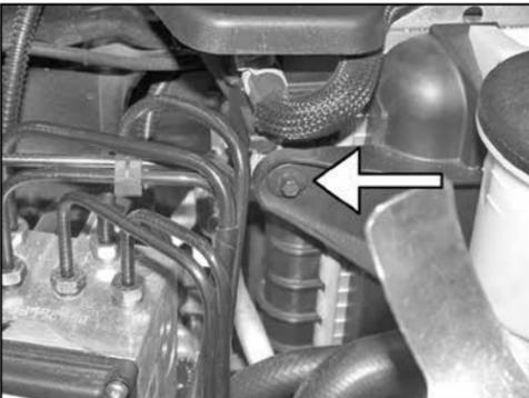
14. Remove the radiator fan shroud mounting bolt shown.
