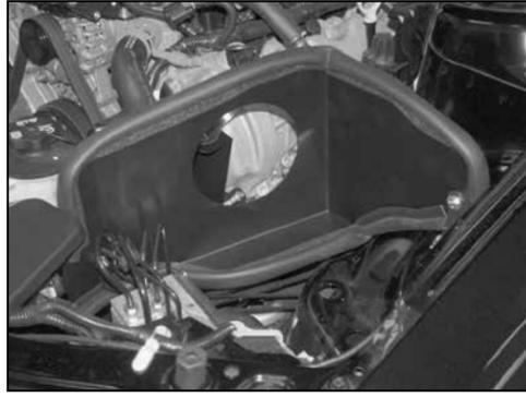
15. Install the heat shield and secure with the provided hardware as shown.
