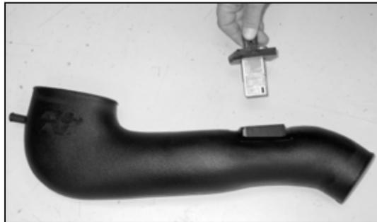
17b. Install the mass air sensor assembly into the K&N® intake tube and secure with the provided hardware.
