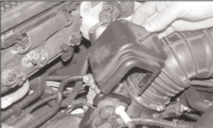
3. Pull up firmly to remove the throttle linkage cover as shown.
