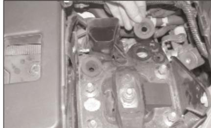
8. remove the rubber grommet from the air box mounting bracket as shown.
