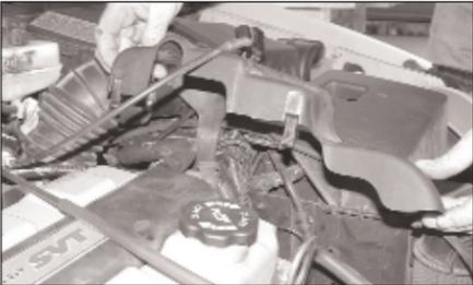
4. Pull up firmly to remove the coil pack cover as shown.
