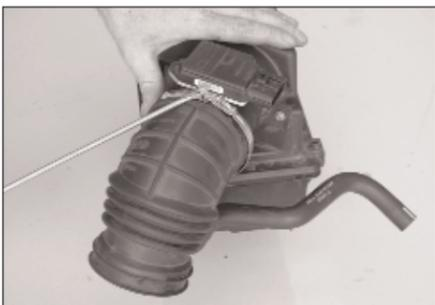
21. Remove clamp that secures the intake tube to the mass air sensor then remove hose.
