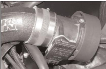
25. Install the mass air sensor assembly onto the intake tube as shown.
