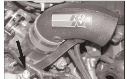
14. Install the new intake tube onto the throttle body, then mount the bracket onto the valve cover with the provided hardware.
