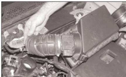
7. Pull up firmly to remove the complete air box assembly from vehicle as shown.
