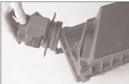
22. Unscrew the mass air sensor from the air box then remove the mass air sensor.
