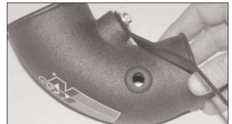
12. Install the provided grommet onto the intake tube as shown.
