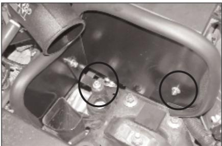
20. Install the heatshield assembly onto the vehicle and then secure to the bumper studs as shown.
