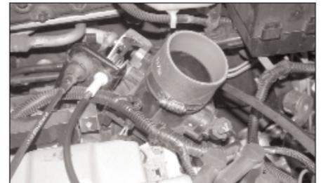
13. Install the silicone hose (08756) onto the throttle body with the provided hose clamps.
