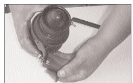
12. Using the hardware provided, attach the short "Z" bracket and twist bracket to the mass air sensor as shown.
