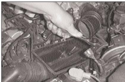
6. Using a 12mm socket, loosen and remove the bolt and the two nuts that hold the airbox base in place.
