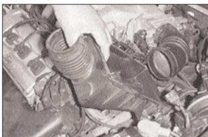
7. Detach the air inlet boot and remove the airbox from the engine compartment.
