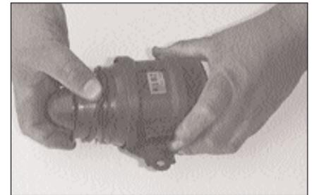
10. Place the provided o-ring into the groove on the mass air sensor as shown.
