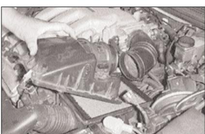
5. Release the airbox clips and remove the airbox lid.
