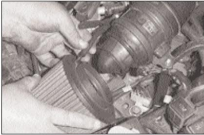
18. Place the air filter in the engine compartment. Insert the vacuum hose with hose mender attached into the small hole located on the element base as shown above.
