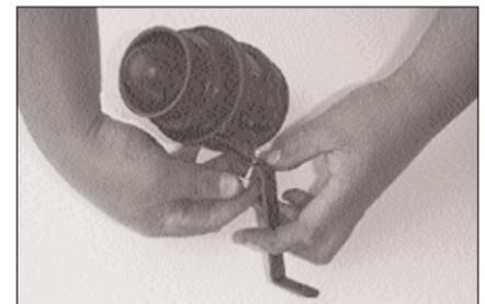
11. Using the hardware provided, attach the short "Z" bracket to the mass air sensor and tighten as shown.
