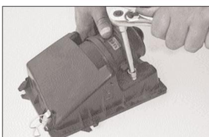
9. Using a 10mm socket, loosen bolts and remove the mass air sensor from the airbox lid as shown.
