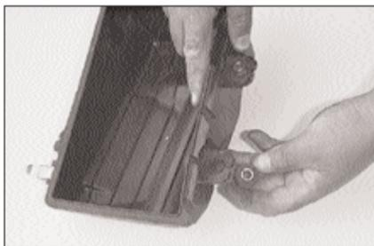
8. Remove one of the factory spacer/grommet from the airbox base as shown and reinstall the factory spacer/grommet onto the stud closest to the throttle body.
