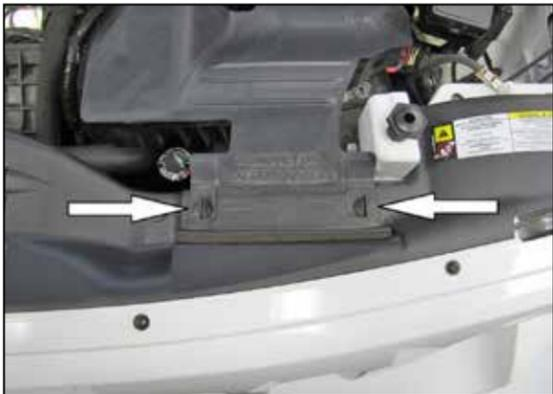
2. Release the two locks securing the fresh air intake scoop and then remove the fresh air intake scoop from the vehicle.
