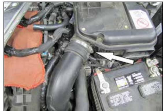
6. Loosen the hose clamp which secures the intake tube to the air box and then disconnect the intake hose from the air box.
