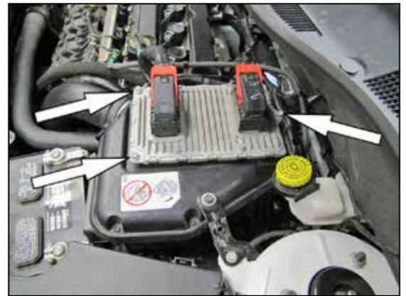
5. Remove the three bolts securing the ECU and ECU ground to the air box lid and then flip the ECU over and lay it on the valve cover.
