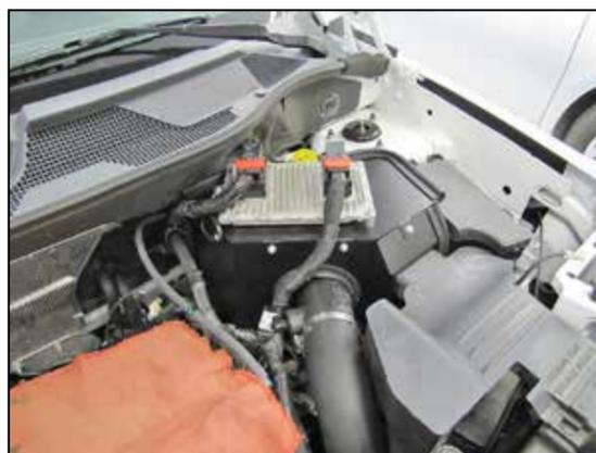
29. Secure the heat shield lid to the heat shield and factory air box mount using the provided hardware. **NOTE: The wiring harness will need to be adjusted to allow the ECU and lid enough movement to be secured onto the heat shield. Disconnect the harness anchors from the attaching posts on the intake manifold, valve cover and engine. After the lid and ECU are secured to the heat shield, adjust the mounts on the harness and resecure the harness onto the valve cover and intake manifold.**
