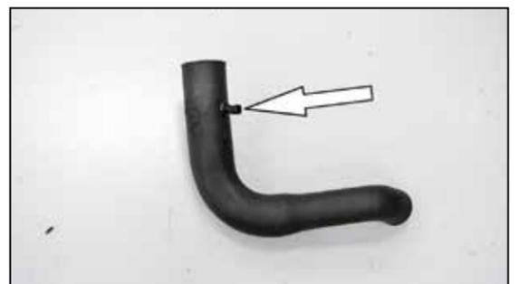
22. Install the inlet air temperature sensor into the grommet installed into the K&N® intake tube.
