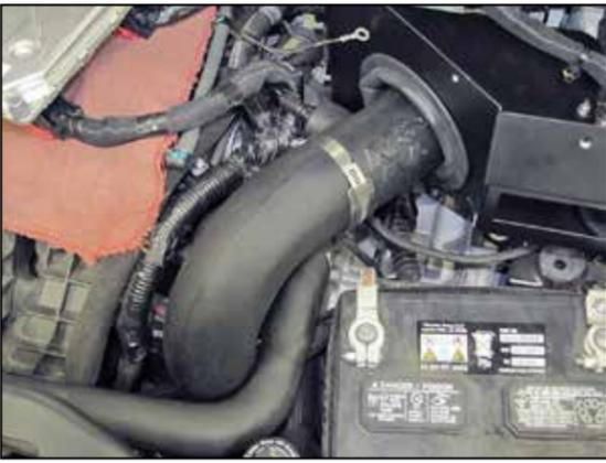
23. Install the K&N® intake tube into the silicone hose at the throttle body and then secure the intake tube with the provided hose clamps.
