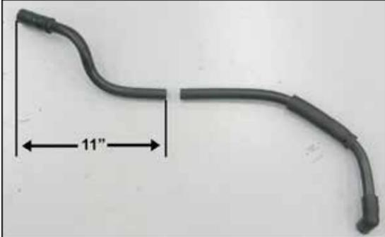
8. Measure 11" from the air filter end of the crank case vent tube and then trim the crank case vent tube as shown.
