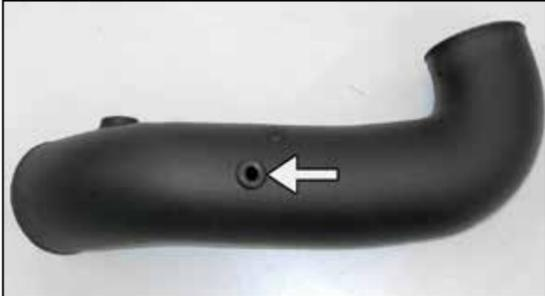
21. Install the provided grommet into the K&N® intake tube as shown.
