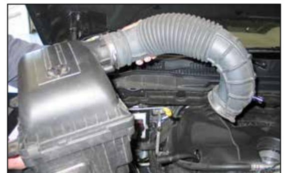
5. Disconnect the factory intake hose from the throttle body, then lift up the air box assembly and remove from the vehicle.
