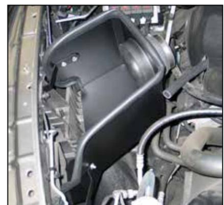
19. Install the heat shield assembly into the vehicle and secure with the bolts removed in steps #17 and 18. Do not completely tighten at this time.
