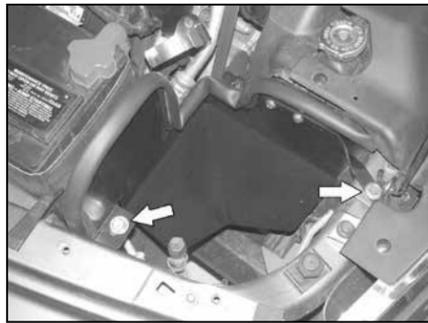
16. Install the K&N® heat shield assembly and secure the mounting bracket to the radiator core support with original bolt removed in step #13. Secure the rear of the heat shield to the 3/8" threaded insert with the provided hardware.
