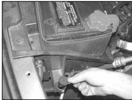
15. Install the 3/8" threaded insert provided into the air box mounting grommet hole vacated in step #14.
