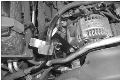
11a. On 2008 and later model year vehicles, attach the tube mounting bracket assembly (070101) to the alternator mounting bolt as shown.
