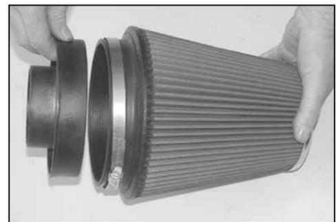
26. Install the provided radius filter adapter into the K&N® air filter and secure with the provided hose clamp.
