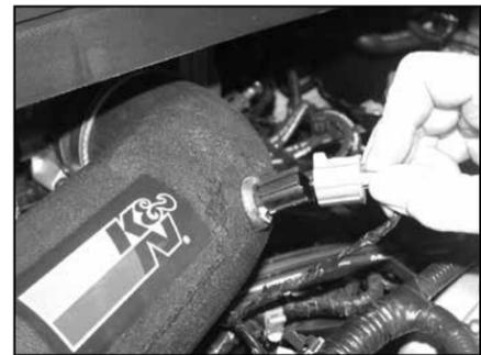
24. Reconnect the temp sensor electrical connection.
