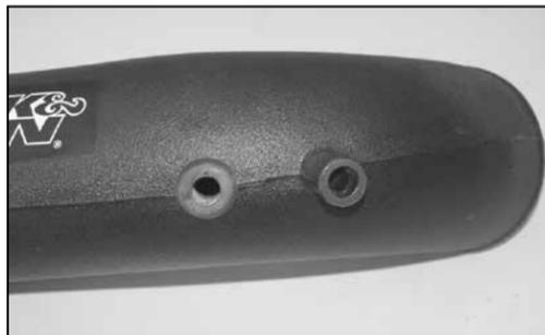
20. Install the provided grommet into the K&N® intake tube as shown.
