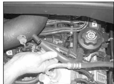
25. Connect the provided silicone hose to the crank case vent on the valve cover, then connect to the K&N® intake tube.
