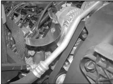
11. On 2007 and earlier model vehicles, install the tube bracket assembly as shown using the hardware provided.
