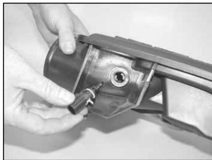
18. Twist the temp sensor counter clockwise to unlock and remove the temp sensor from the resonator.
