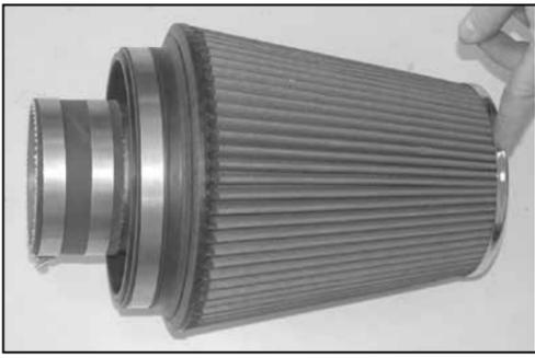
27. Install the silicone hose (08630) onto the K&N® air filter assembly and secure with the provided hose clamp.
