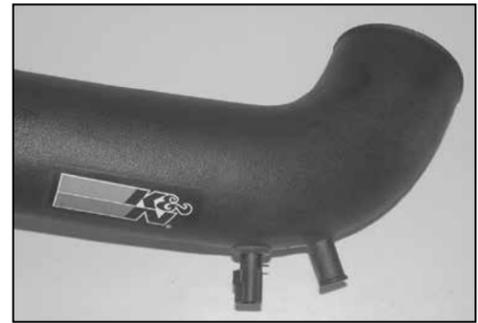
21. Install the air temp sensor into the K&N® intake tube as shown.
