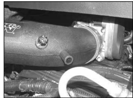
22. Install the intake tube onto the throttle body and secure with the provided hose clamp.
