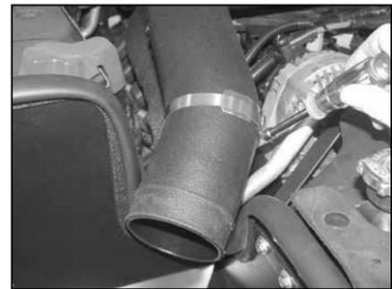
23. Using the provided hose clamp, secure the K&N® intake tube to the saddle bracket assembly as shown.
