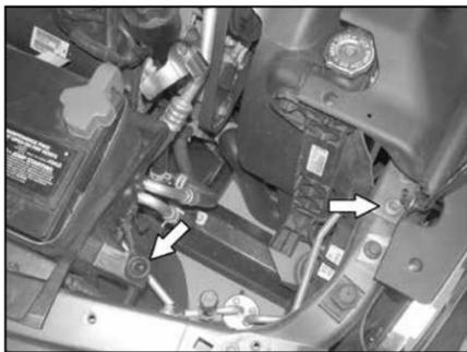
14. Remove the core support mounting bolt shown with a 13mm wrench, and pull out the stock air box mounting grommet shown.
