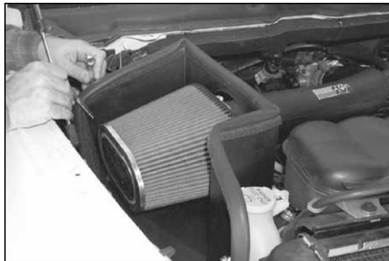
33. Align the heat shield for best clearance then tighten all the brackets.
