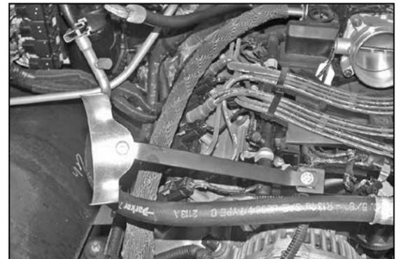
21a. On vehicles equipped with an air injection valve, secure the tube mounting bracket assembly (#07192) to the resonator mount on the intake manifold. Secure using the provided 6mm hardware as shown.
