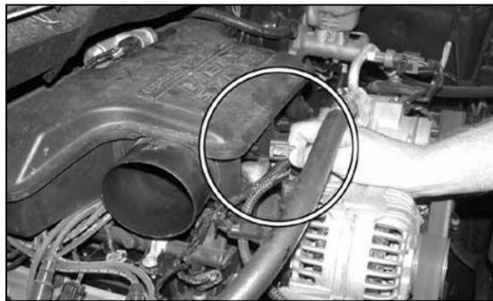
4. Disconnect the air temp sensor electrical connection as shown.
