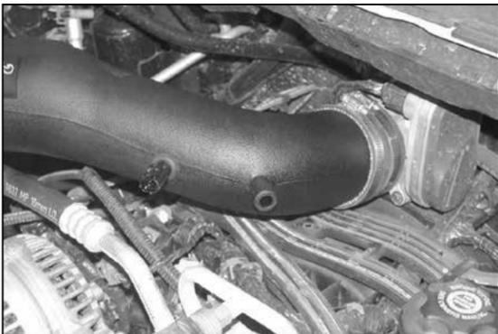
28. Install the intake tube onto the throttle body with the provided hose clamps.
