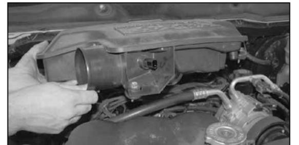
7. Remove the resonator box from vehicle.
