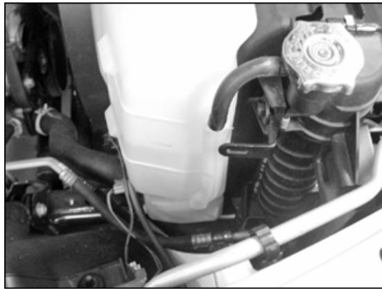
16. Install the "L" bracket (26607) onto the fan shroud with the provided 8mm bolt and washers.
