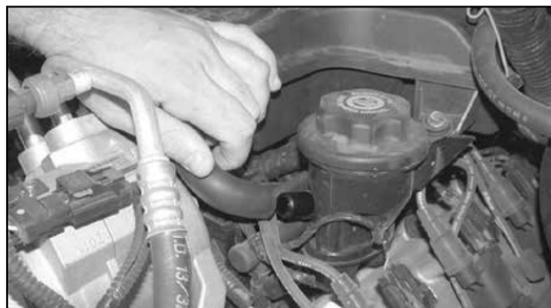
6. Disconnect the crankcase vent hose from oil fill as shown.
