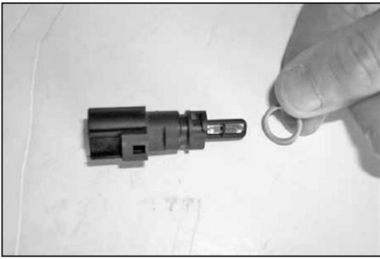
24. Remove the O-ring from the air temp sensor as shown.
