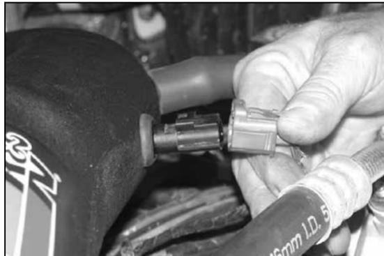
31. Reconnect the air temp electrical connection.
