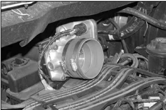
27. Install the provided silicone hose (08630) onto the throttle body with the provided hose clamps.
