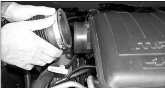
2. Loosen the hose clamp that connects the intake tube to the resonator box then remove the intake tube.
