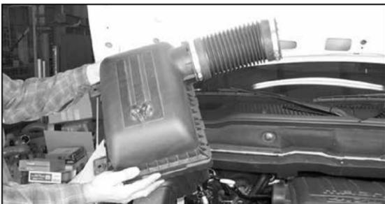
3. Lift up firmly to release the airbox from mounting studs, then remove completely.
