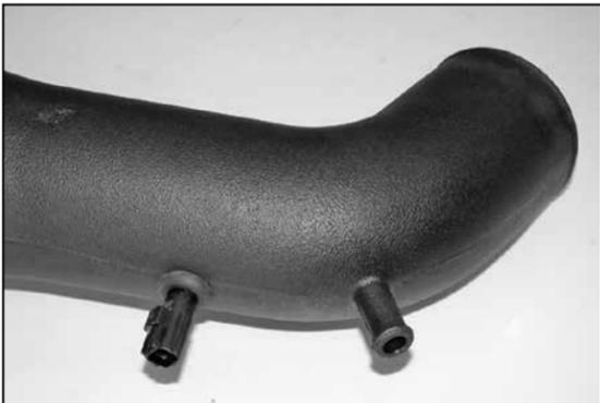
26. Install the air temp sensor into the new intake tube as shown.
