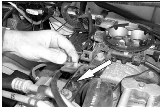
5. Remove the stock grommet and the stock plastic locating pin as shown.
