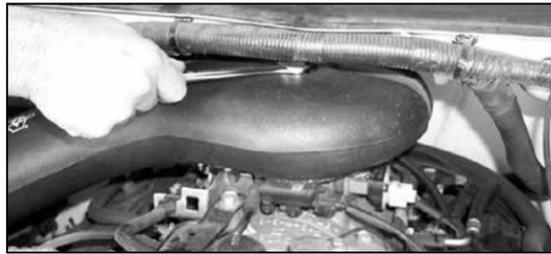
36. Position the K&N intake tube onto the throttle body, then, secure the K&N intake tube to the throttle body with the nut extension as shown.
