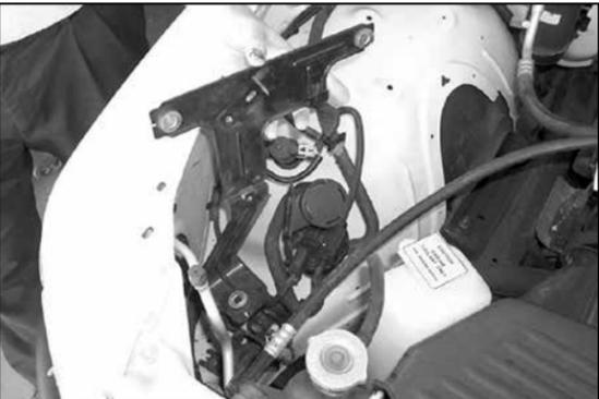
10. Remove the EVAP assembly bracket from the vehicle as shown.
