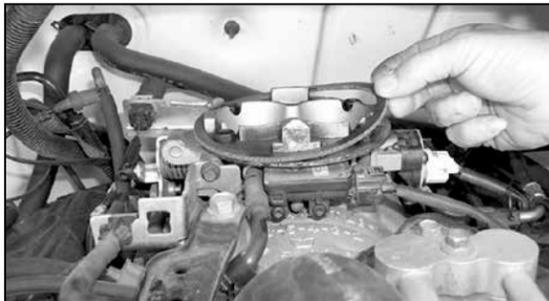
18. Replace the stock throttle body gasket with the provided K&N® gasket as shown.
