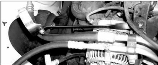
30. Install two washers onto the stock air cleaner mounting stud, then, install the saddle bracket assembly onto the stud and secure with the provided hardware as shown.
