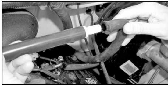
33. Assemble the provided hose mender and the provided silicone hose as shown, then connect it to the stock crank case vent hose as shown.
