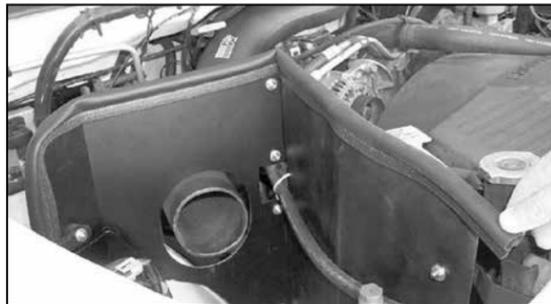
38. Install the provided edge trim onto the K&N heat shield as shown.
