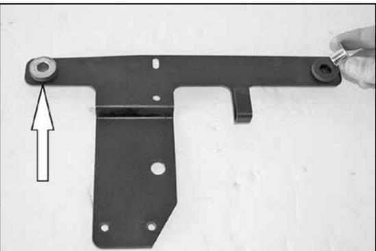
11. Remove the two upper stock metal stand-offs and the stock grommets from the stock EVAP assembly bracket and install them into the new K&N® EVAP assembly bracket as shown.
