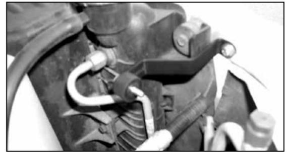
21. Secure the "Z" bracket to the radiator core support using the provided hardware as shown.
