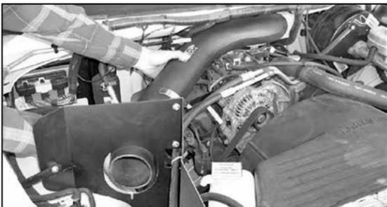
32. Install the K&N intake tube into the hole on the K&N heat shield, then, line up the other end with the throttle body as shown.
