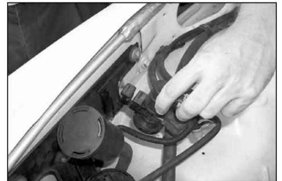
6. Remove the EVAP canister purge solenoid from the EVAP assembly bracket located on the inner fender as shown.
