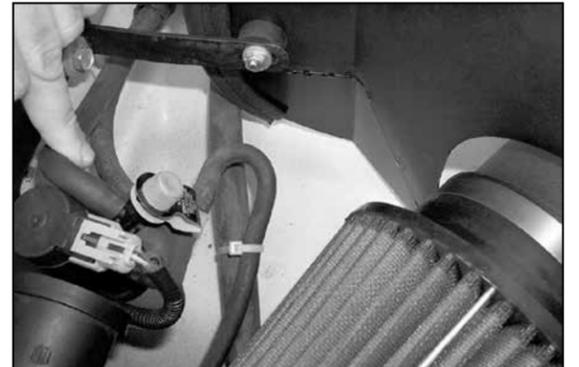
40. Using the provided zip tie, bundle up the EVAP assembly vent hoses as shown.
