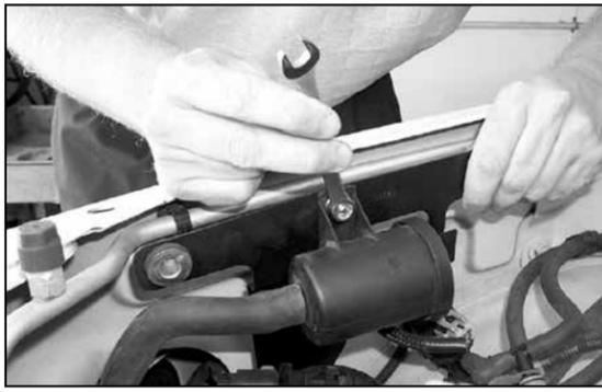
14. Install the EVAP canister vent onto the EVAP assembly bracket using the hardware provided as shown.
