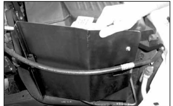
24. Install the first half of the heat shield into the vehicle and secure it to the "Z" bracket using the provided hardware as shown.
