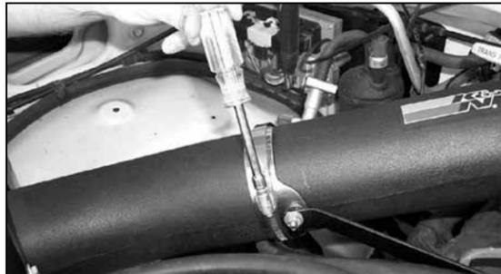
37. Secure the K&N intake tube to the saddle bracket using the provided hose clamp as shown.
