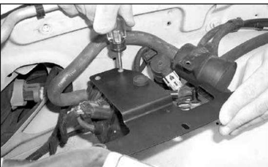
13. Install the EVAP canister onto the K&N® EVAP assembly bracket using the original screws removed in step 9.
