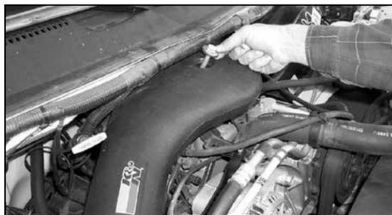
35. Install the nut extension and the provided washers into the hole on the K&N intake tube as shown.
