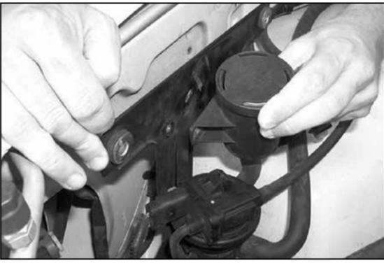
8. Loosen and remove the EVAP canister vent from the EVAP assembly bracket as shown.
