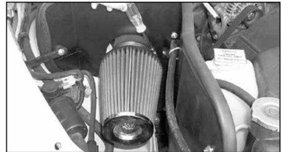
39. Install the K&N Air Filter onto the K&N intake tube and secure it with the provided hose clamp as shown.
