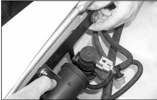
16. Install the purge control solenoid onto the K&N® EVAP assembly bracket as shown.
