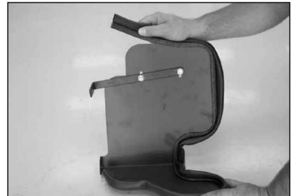
7. Install the trim seal to the heat shield as shown. Trim as needed.
