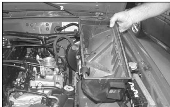
5. Loosen and remove the two bolts, and one nut to remove the lower air box assembly.
