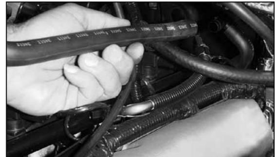
9. Detach the OE crankcase vent hose from the "T" fitting.
