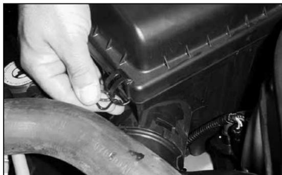
4. Release the 4 over center clips that retain the airbox top to airbox base.
