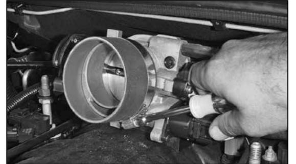
21. Attach the silicone hose to the throttle body using a hose clamp provided.
