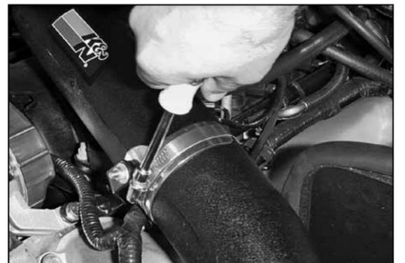
23. Secure the intake tube to the saddle bracket using the hose clamp provided.
