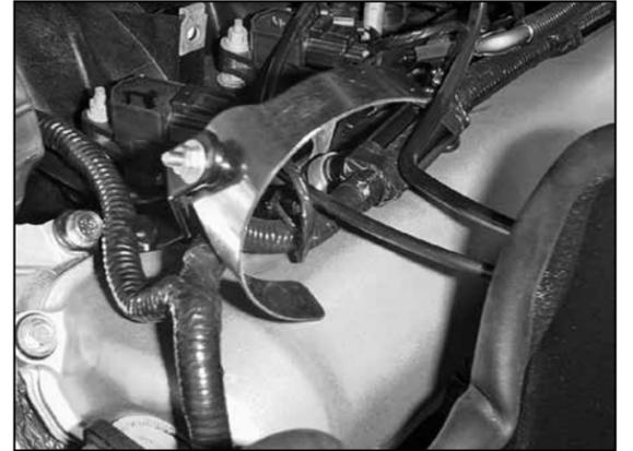
20. Attach the saddle bracket assembly to the alternator using the bolt removed in the previous step.
