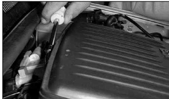
6. Loosen the hose clamp on the intake tube at the throttle body.
