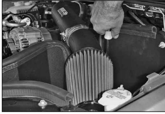
28. Install the K&N® Air Filter onto the intake tube and tighten hose clamp provided.
