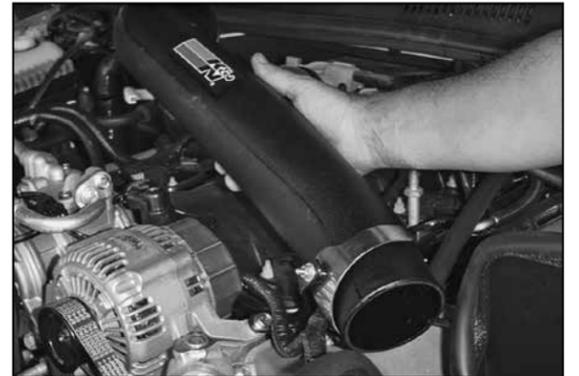
22. Install the K&N® intake tube.
