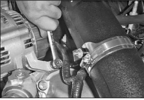
25. Tighten the alternator retaining bolt.
