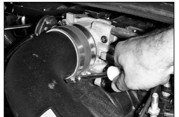
24. Tighten the hose clamp on the silicone hose at the intake tube.
