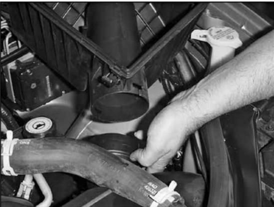
11. Detach the air inlet duct from the airbox base and remove the airbox base.
