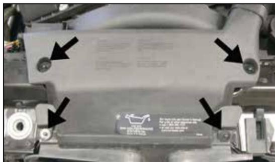
3. Pull up on the four fresh air duct-retaining pins to release them from the radiator core support.
