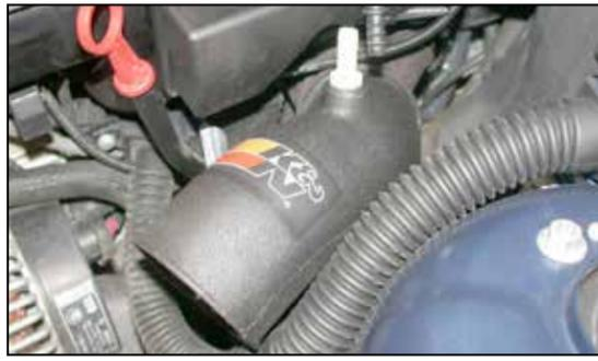
13. Install the K&N® intake tube into the factory lower intake hose and secure with the factory hose clamp.
