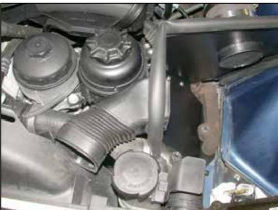
27. Install the factory fresh air tube into the heat shield as shown.
