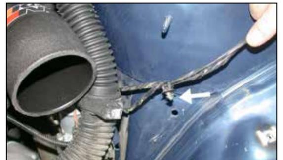
21. Using a pair of pliers, carefully remove the wiring harness retaining clip from the inner fender as shown.
