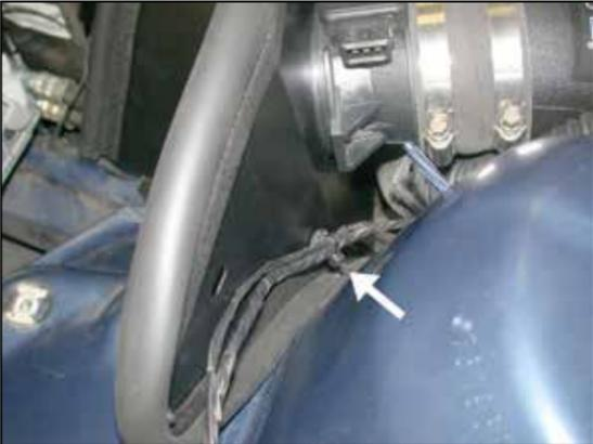
25. Secure the wiring harness clip removed in step #21 to the heat shield as shown.
