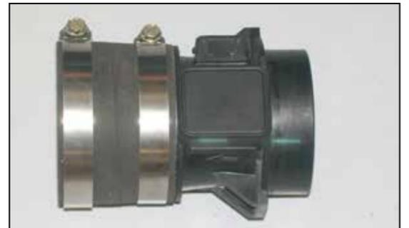
20. Install the silicone hose (08690) onto the mass air sensor and secure with the provided hose clamp.
