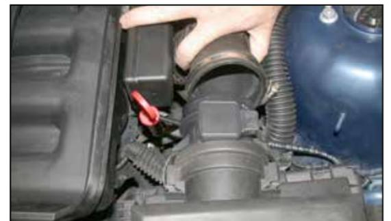
5. Loosen the hose clamp that secures the intake tube to the mass air sensor and then disconnect the intake tube from the mass air sensor as shown.
