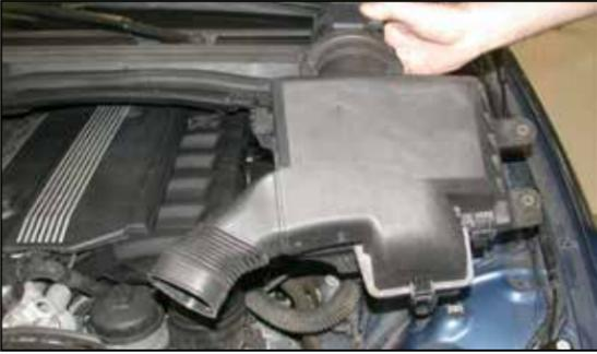
8. Lift up and remove the air box from the vehicle.
