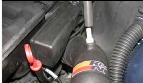
29. Using the supplied silicone hose, attach the factory vent hose to the npt fitting on the intake tube.
