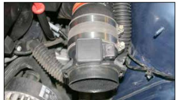
22. Install the mass air sensor assembly onto the K&N® intake tube and secure with the provided hose clamp.
