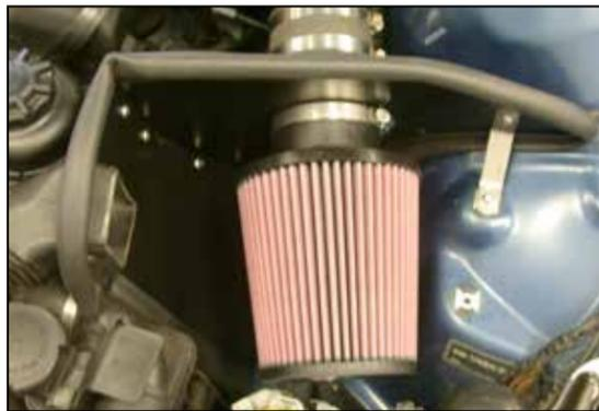
31. Install the air filter and secure with the hose clamp provided.
