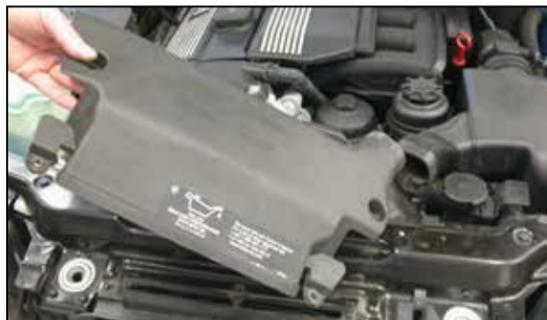
4. Lift up and remove the fresh air duct from the vehicle as shown.
