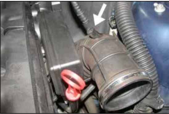
9. Disconnect the vent tube from the factory intake tube as shown.
