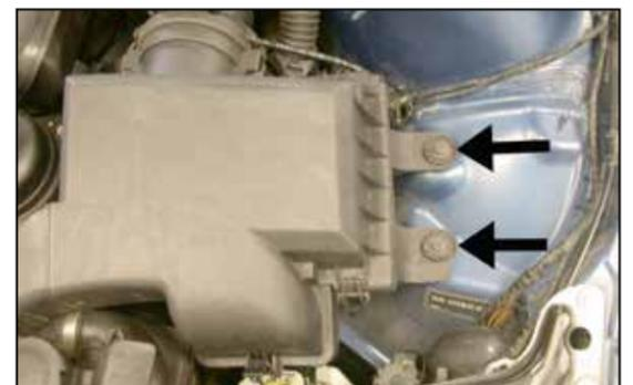
6. Remove the two factory air box mounting bolts shown.
