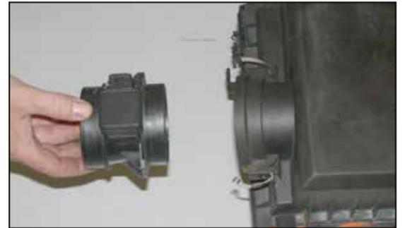
19. Release the two clips that secure the mass air sensor to the air box, then remove the mass air sensor as shown.
