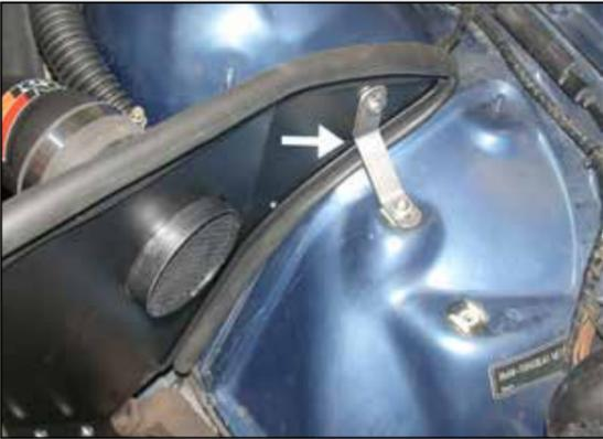
26. Install the provided bracket onto the heat shield and inner fender with the provided hardware as shown.
