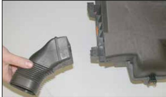
14. Remove the factory fresh air hose from the air box as shown.
