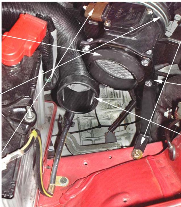
**1.** Fit the adaptor plate to the MAS using the gasket, screws, nuts and washers supplied.
