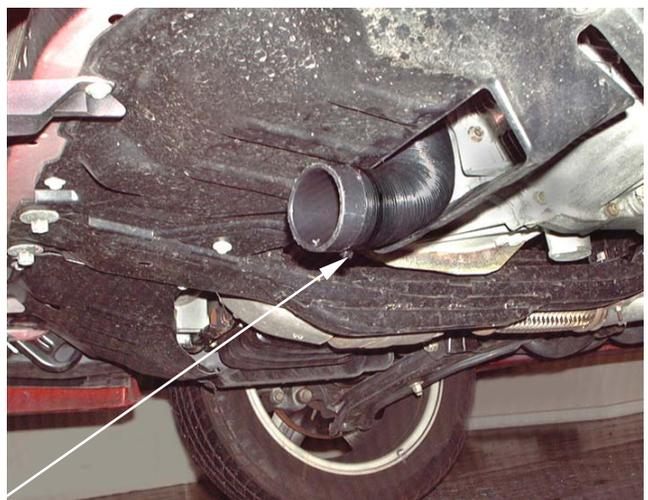
Feed the flexi cold air hose down and through the gap in the undertray. Drill two 3mm holes in the undertray and secure the end of the flexi cold air hose to it using a long plastic tie supplied.
