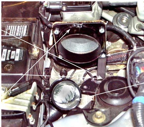
4. Refit the MAS assembly onto the intake hose and secure the original hose clip.
