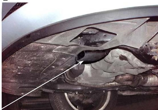
Taking all of the necessary safety precautions as per the manufacturers instructions, raise the front of the car. Pierce / drill two 3 mm holes in the under tray and secure the rubber scoop to it using a long plastic tie supplied. Insert the flexi cold air hose into the rubber scoop, secure the rear of the scoop / hose with a long plastic tie supplied
