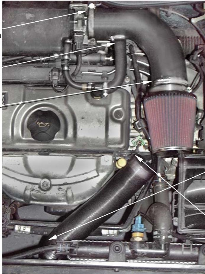
5. Fit the filter assembly into the new intake hose and firmly tighten the studded hose clip, rotate the filter until the K&N logo is straight then give the clip one full turn (360 degrees) **no more. Do not overtighten the clip.**
