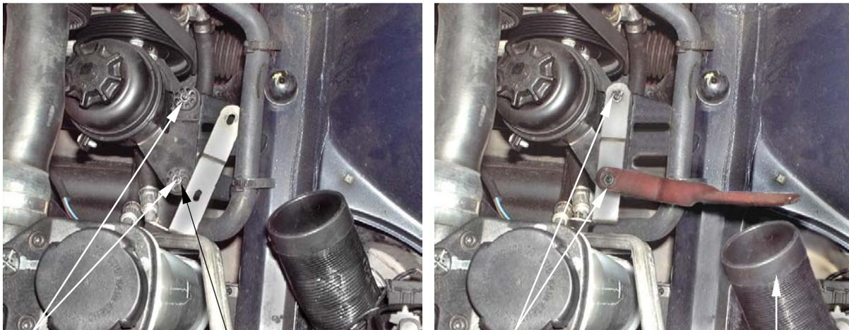
1. Remove the 2 nuts securing the PAS reservoir and air conditioning pipes to the chassis leg.
