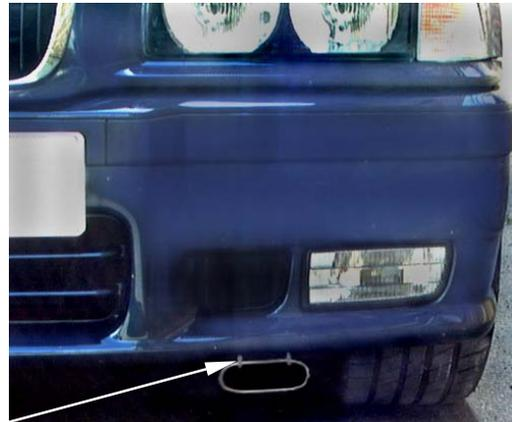
Taking all of the necessary safety precautions as per the manufacturers instructions carefully raise the front of the car. Unclip and remove the under tray side trim. Once the trim has been removed, refit the 2 securing screws to the under tray / wheel arch liner. Pierce drill two 3 mm holes in the front lower spoiler trim and secure the new cold air scoop to it using a long plastic tie. Secure the rear of the scoop to the wheel arch liner.
