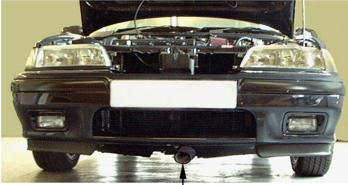
Feed the flexi cold air hose down to the centre of the front lower spoiler. Pierce a 3mm hole in the bottom of the cold air hose and attach the hose to the front towing eye using the plastic tie provided. Ovalise the end of the cold air hose to increase ground clearance.
