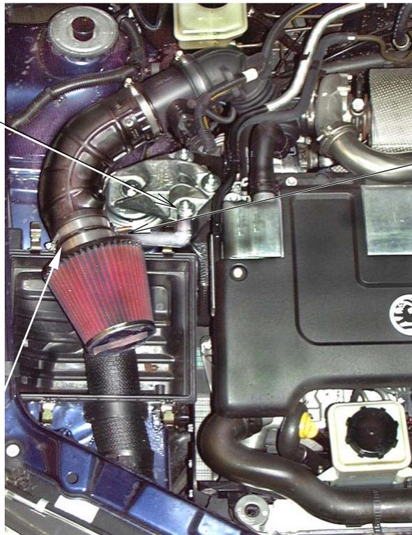
1. Remove the nut from the engine mounting front stud. Fit the new bracket to the stud using the original nut.
