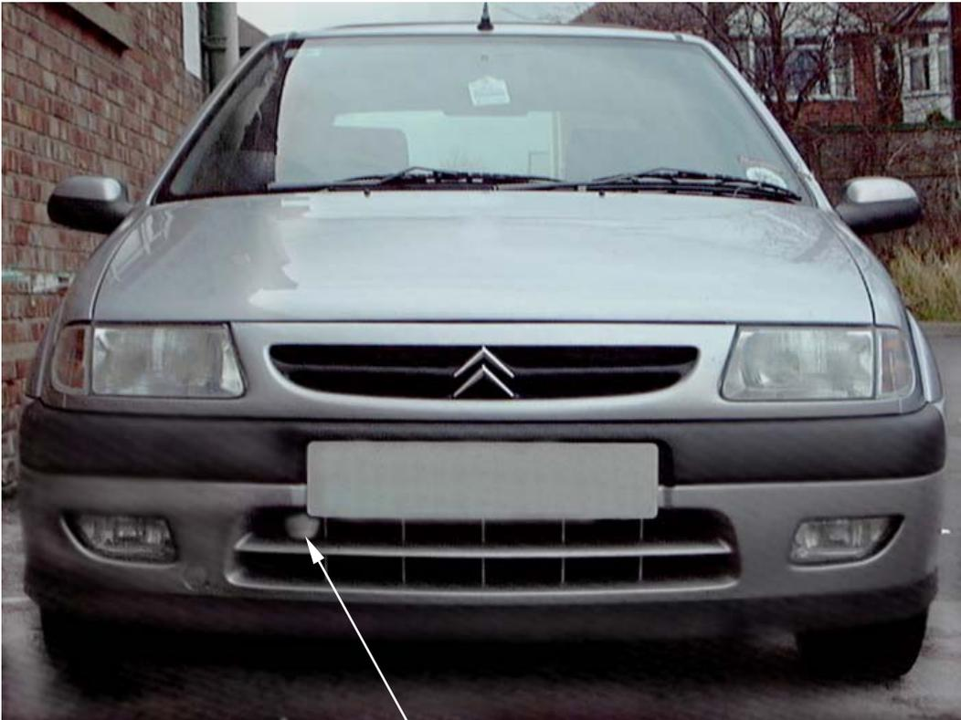
Feed the flexi cold air hose down to the lower grille. Pierce / drill a 3mm hole in the end of the flexi cold air hose and attach it to the grille using a plastic tie supplied.
