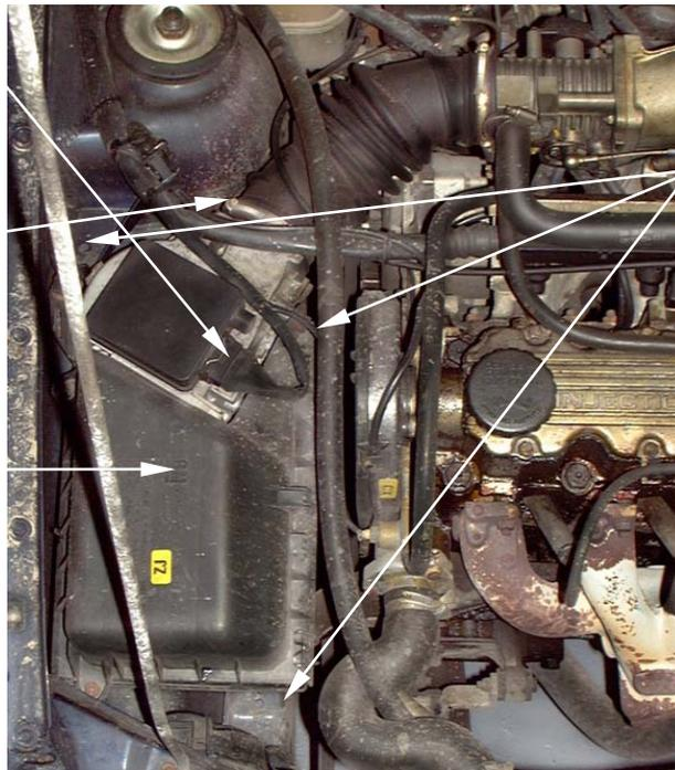
4. Release the 3 nuts securing the air box base to the inner wing. Lift out the air box base from the mountings and remove from the vehicle.
