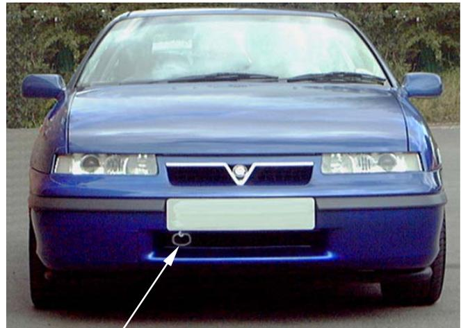
Feed the flexi cold air hose to the front grille and secure with a long plastic tie supplied.
