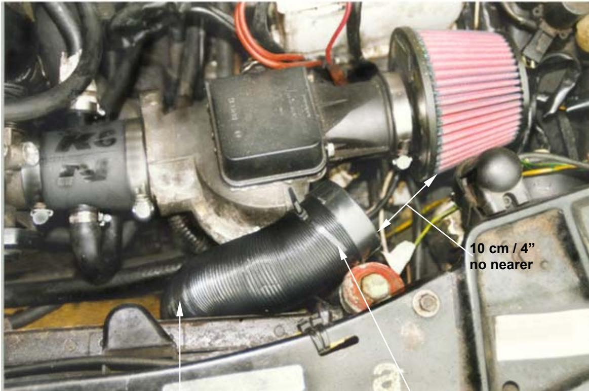
1. Carefully lengthen the flexi cold air hose to approx. 84cm / 33". Feed the flexi cold air hose down between the engine and radiator to the L.H.S. tow hook. Ovalise the end of the hose and tie to the rear section of the tow hook using a long plastic tie. Ensure the end of the hose is in the air stream.
